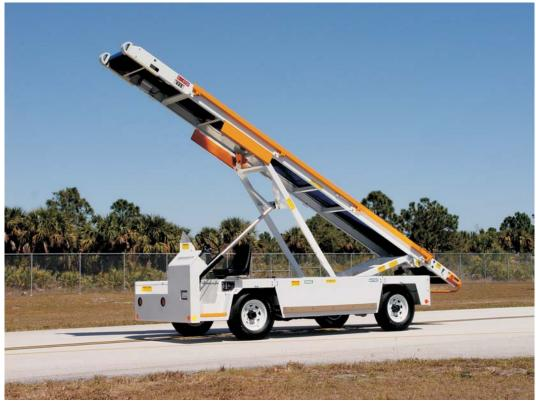
The Phoenix MBL is a mobile baggage loader. It is designed for the rugged nature of airport ramp operation. The chassis is a heavy duty formed chassis. The conveyor bed is also designed to withstand the rough airport environment.
