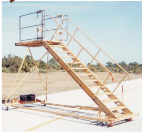
The Phoenix FCS 104 Fixed Crew Stair is a lightweight stair for accessing aircraft for crewmembers. The FCS104 can be maneuvered by one person and has an easily controlled braking system. The FCS 104 has adjustable handrails to allow for aircraft door opening and a non-marring front bumper. The stair treads have a non-skid surface. The FCS 104 is designed for ease of maneuvering and also can be easily collapsed for shipping.
